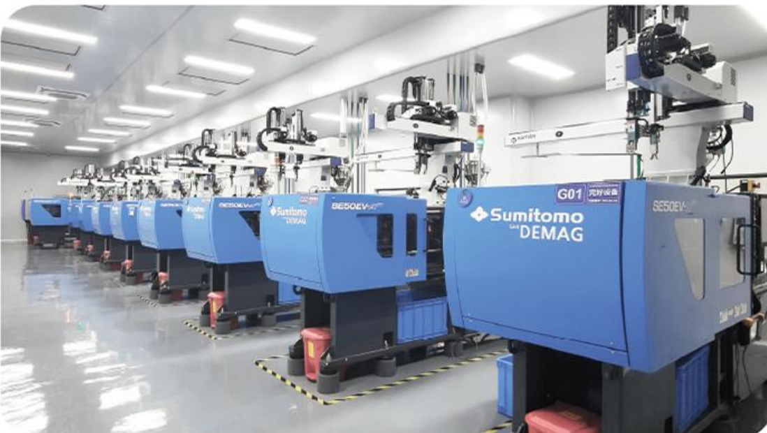
▲ Cleanroom Molding Zone(Class 100,000) SE50-100 series
